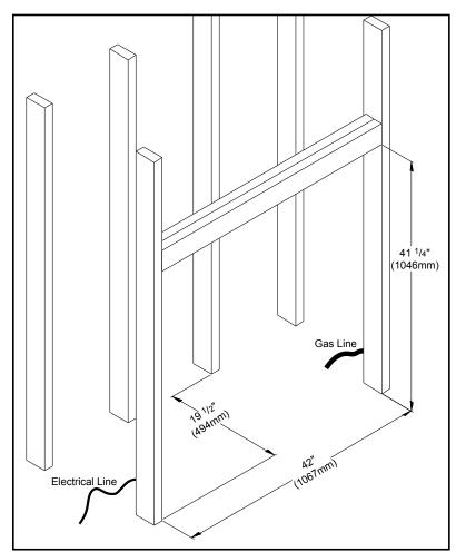
Figure 10. Dimensions for Framing the Firebox.
